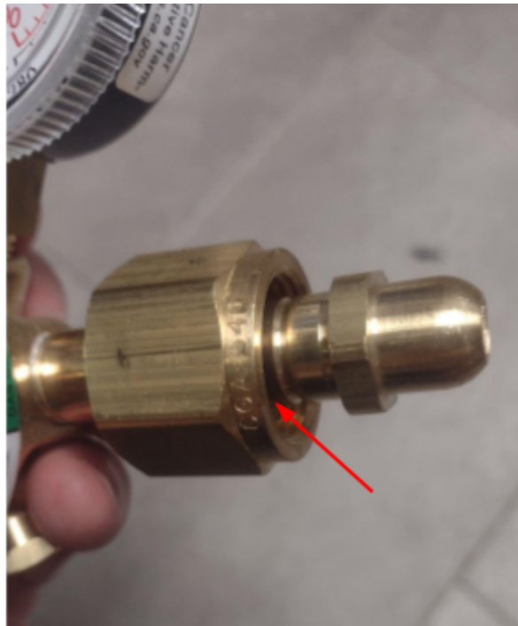
Note the CGA540 markings on the nut
