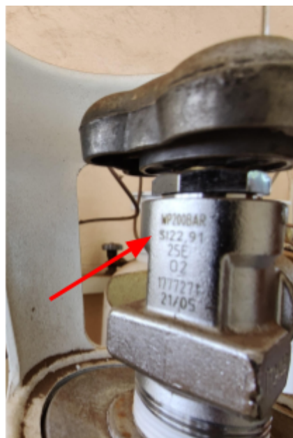
"SI 22.91" refers to the outside diameter and threadform of the outlet thread on the valve. British valves do not use this designation.
