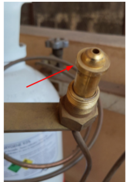
Note the raised ridge on the nipple.
