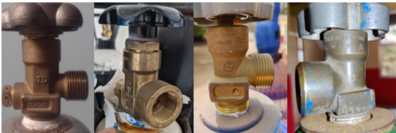
Different bullnose valves for oxygen. Despite some looking nearly identical, all of these valves are from different non-compatible standards. Equipment that connects to one valve will not fit on the others valves.
